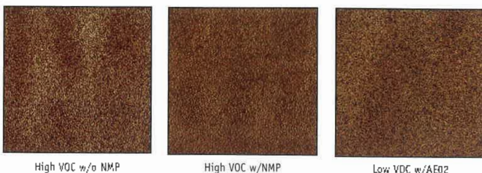
Figure 4—AFM micrographs of films prepared from Polymer Emulsion A. Films containing the AE02 surfactant were smoother than higher VOC analogs.
