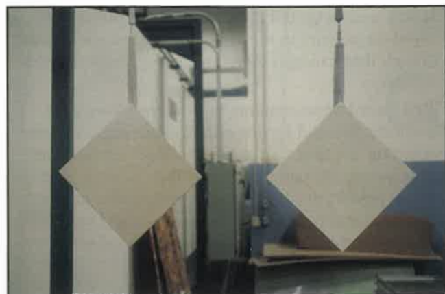
Figure 1—The primed fiberboard was grounded via a wire hanger inserted into a hanger hole on the corner of MDF and hooked onto a flight bar of the powder line chain.
